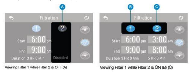
Press "1" (B) to view Filter 1. Press "2" (C) once to view Filter 2. Press "2" again to turn Filter 2 ON or OFF.
