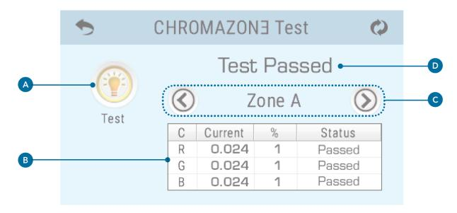
CHROMOZON∃™ Test tests the electrical load of all the LEDs in all zones connected to CHROMOZON∃™ (E).
